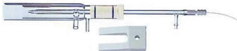
These above conditions are only for reference and may not be ideal for all instruments. Please also note that the Vulkan tip should remain at least 5mm recessed from the inner tube of the torch in order to prevent damage from the heat of the plasma.
