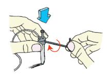
6. Ensure that the indentations in the nebulizer body line up with the threaded holes. Pushing down on the fitting, tighten the 2 grub screws firmly.
