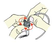
5. Holding the nebulizer in the left hand again, insert the new sample tube by twisting left to right and pushing it in gently, until it stops.
