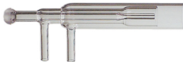
Single-Piece Quartz Torch with 2mm Bore Injector
