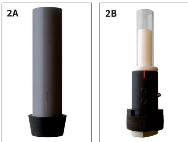
Figure 2. The radial D-Torch ceramic outer tube (2a) and the radial D-Torch, with a quartz outer tube to show the geometry of the intermediate tube (2b).
