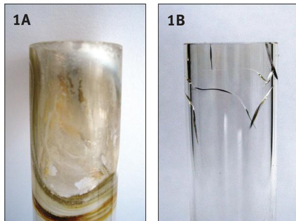
Figure 1. Examples of devitrification (1a) and premature failure (1b) of quartz ICP torches.
