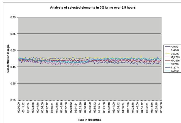
Figure 4. A plot of the stability run with the radial ceramic D-torch continuously analyzing a 3 % sodium chloride solution spiked at 0.5 mg/L with the elements of interest.
