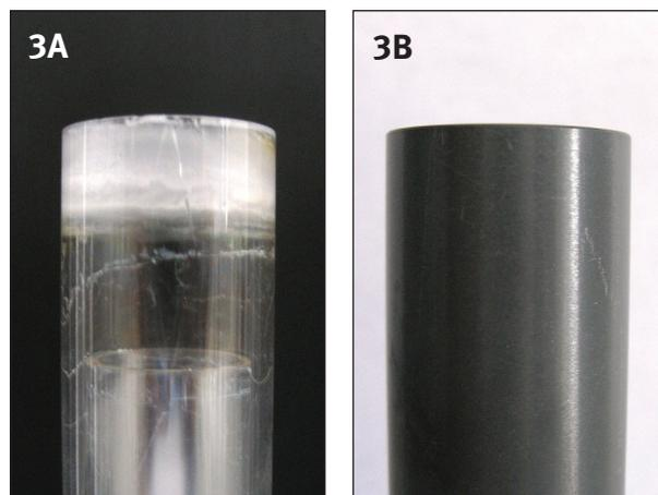
Figure 3. Quartz torch (3a) and the radial Ceramic D-torch (3b) after 10 hours continuous analysis of 10 % sodium chloride solution (after cleaning and drying).
